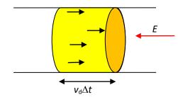
The length of the cylinder is  $v_d \Delta t$  where  $v_d$  is the drift speed of electrons. In time  $\Delta t$  every electron in the shaded cylinder will pass through the cross-sectional area of the cylinder (shaded orange). The number of electrons in the shaded cylinder is  $N = nV = nAv_d\Delta t$ . The charge in the cylinder is then  $\Delta Q = eN = enAv\Delta t$ .
